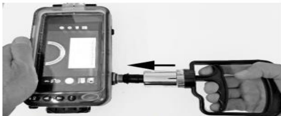
Hand pump pressed against vacuum check port
